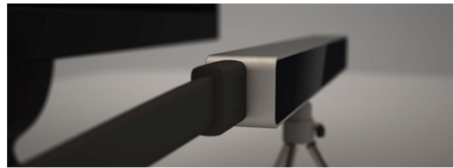
Fig. 1 Eye Tribe tracker with USB plug in front of a computer monitor
